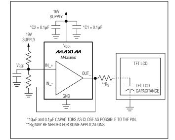
Figure 2. Typical TFT-LCD Backplane Drive Circuit
