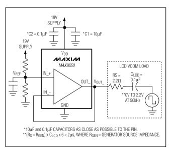
Figure 1. Settling Time Test Circuit
